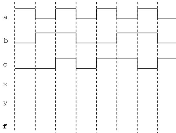
c) The following is the timing diagram of a logic circuit with 3 inputs. Sketch the logic circuit that generates this waveform. Then, complete the VHDL code (using VHDL signals is optional). (8 pts)
